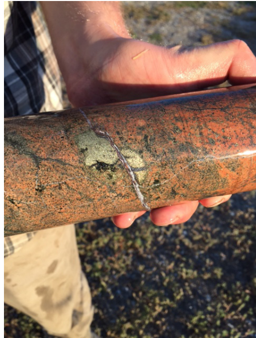
Fig. 5. Copper King copper-gold project, 20 kilometres west of Kamloops. Offset sulphide lens and quartz veinlet in brecciated Cherry Creek monzonite, a phase of the Iron Mask batholith (Image courtesy of Copper King Exploration Ltd.).
