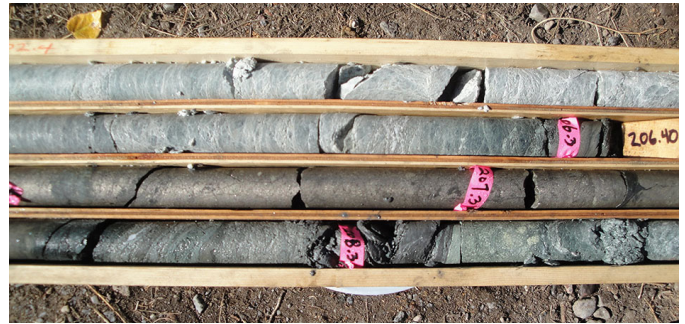
Fig. 7. Redhill volcanogenic massive sulphide project. Massive sulphide layer (between pink flagging) at the Alpha zone, 15 kilometres south of Cache Creek (Image courtesy of Troymet Exploration Corp.).
