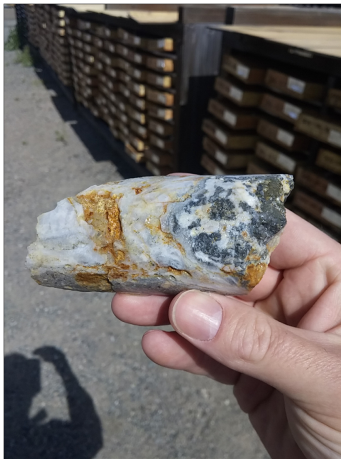
Fig. 4. Shovelnose gold project. Westhaven Ventures Inc. explored low-sulphidation epithermal gold systems south of Merritt. This sample had ~16 grams per tonne gold and ~30 grams per tonne silver (Image courtesy of Westhaven Ventures Inc.).
