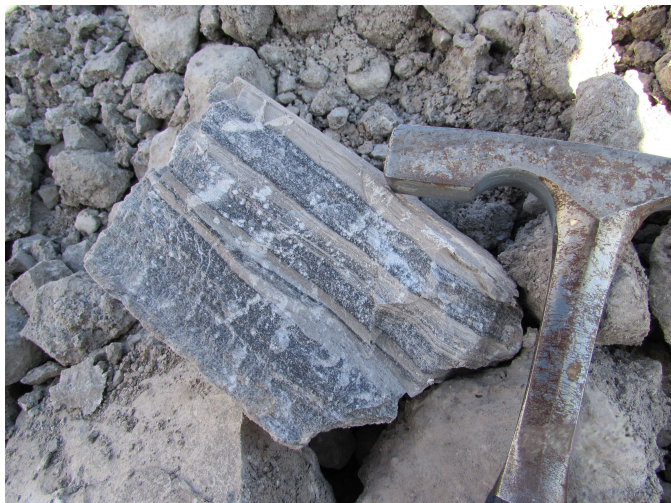
Fig. 16. Inter-bedded gypsum and finely laminated mudstones in the middle Devonian Burnais Formation. Gypsum is produced from the Burnais formation at the Elkhorn and 4J mines, with a new mine development proposal in EA for the Kootenay West mine.
